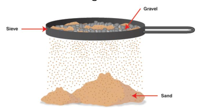
The sieve has very small holes. Coarse particles of sand are separated or broken up by grinding against one-another and the screen openings.
