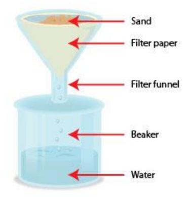
The mixture of sand and water is poured into the filter funnel, which is lined with filter paper. The water can pass through the paper to collect in the beaker. The sand particles cannot pass through the filter paper and collect in the filter funnel.
