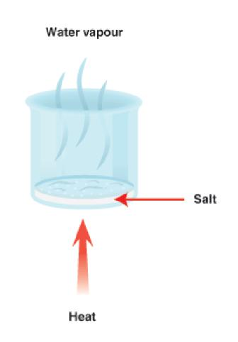
If we collect the water vapor that evaporates we can cool it to form water again.
